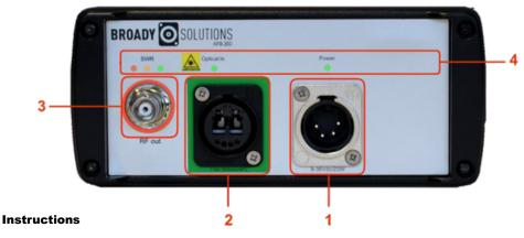
1 - Power : 9-36Vdc-20W linear power supply or battery Consumption 800 mA XLR4 Wiring : 1 - / 4 +
